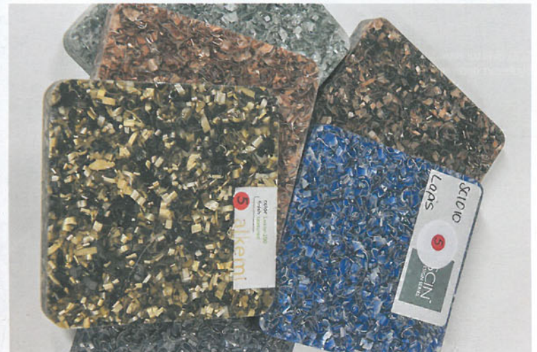
Alkemi is a recycled material made of scraps of waste aluminium flake, solid surface scrap and recycled acrylic, which can be used for horizontal and vertical decorative interior surface applications
