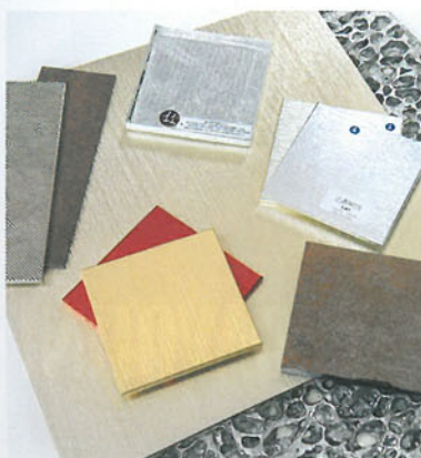
Alusion cellular aluminium foam material forms the backdrop to Alulife recycled aluminium tiles and Textilglass fabric behind glass from Bluestein
